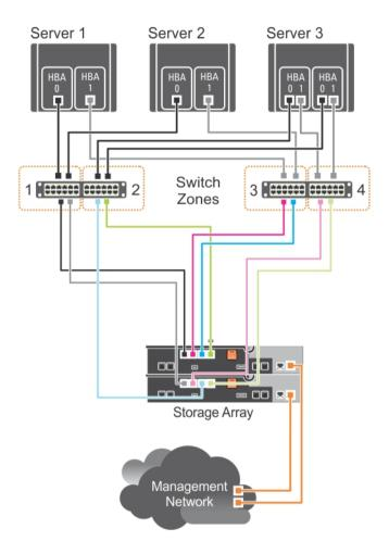
Figure 1. Example of Switch Zoning on SAN on an MD38xxf-series Fibre-Channel Storage Array
